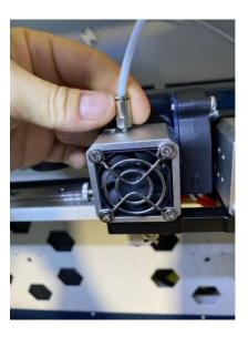
2) Unscrew the tension nut so that the spring is fairly loose. **Do not loosen it so much that the nut** comes off of the screw.
