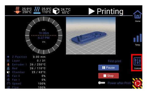
3) Click **Babystep** and use the up and down arrows to adjust the nozzle gap. **START WITH THE SMALLEST INCREMENTS AT FIRST. THERE MAY ALSO BE A DELAY IN THE ADJUSTMENT, SO BE PATIENT.**
