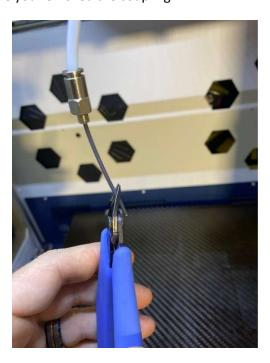
6) Press down firmly on the filament and insert it about 1" (you may have to press it in a couple of times) into the hole.
