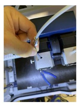
7) Retighten the tension screw on the left a fair amount so that the spring is semi tight. **It does not have to be super tight**. Typically, an 1/8-inch (3mm) gap is a good place. Tug on the filament lightly and you should feel some resistance. This is normal, it means that the extruder is gripping the filament, which is what we want.
